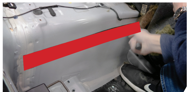
RECOMMEDND LOCATION TO PLACE BOOM MAT TAPE DAMPING MATERIAL ON PASSENGER SIDE TRANS TUNNEL PASSENGER SIDE SHOWN (VIEW FROM PASSENGER DOOR)
